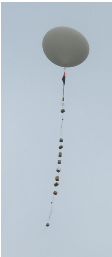
Figure 4.4: Latex sounding balloon launch with multiple student payloads.
