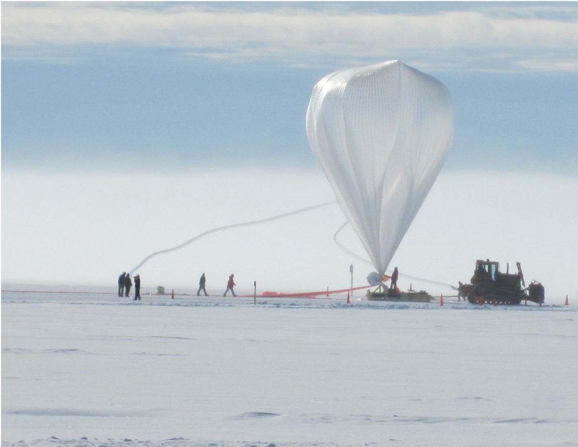
Figure 2.2: Balloon inflation for the LDB Super-Trans-Iron-Galactic Element Recorder ( SuperTIGER ) launch in 2013.
