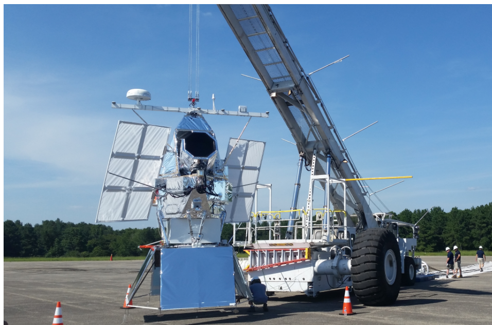
Figure 2.19: SuperBIT is shown on the launch pad in Palestine. During a series of test flights since 2015, the SuperBIT payload has demonstrated wide-field, diffraction limited imaging using a 0.5 meter telescope. SuperBIT is the first instrument to demonstrate sufficient 3-axis pointing stability to enable diffraction limited long exposures (up to 30 minutes) over a large field of view.
