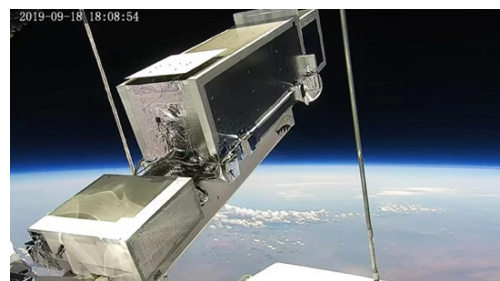
Figure 2.30: The BITSE coronagraph is pointed toward the Sun during its September 2019 flight.
