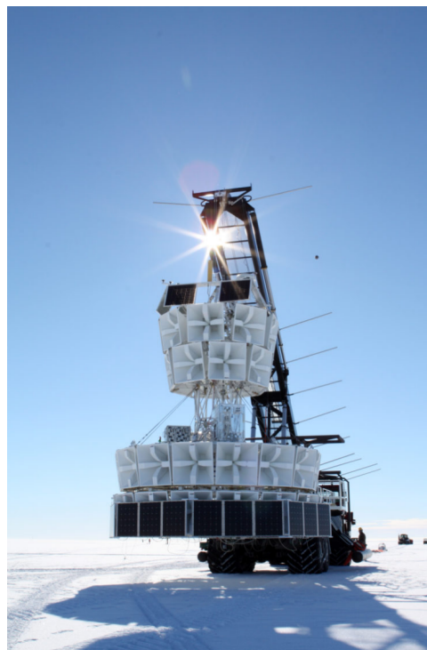
Figure 2.5: The 8-meter high ANITA-III payload suspended from the LDB launch vehicle during launch preparations in 2013.
