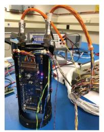
Sub-payload control card bench testing
