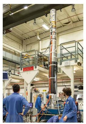
Micro-X on the vibration table during pre-flight testing.
