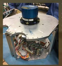
The NSROC developed Tern INS was flown operationally for the first time on 46.021 UO in 2018. The system is designed to generate high quality, reliable body rate and acceleration measurements, attitude propagation, and navigation solutions.
