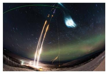
Composite time–lapse photograph of the three Super Soaker rockets launched from the Poker Flat Rocket Range in Alaska on January 26, 2018. The green line in the upper right is the Rayleigh lidar beam. The bright white feature is part of the TMA tracer trail.
