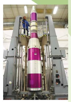
NSROC Testing and Evaluation Lab intern with an ASPIRE payload on the balancing table.
