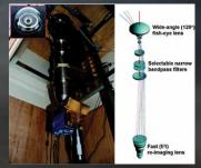
Advanced Mesospheric Temperature Mapper (AMTM) The AMTM is an infrared digital imaging system that measures selected emission lines in the mesospheric Hydroxyl (OH) (3,1) band (at approximately 1.5 µm) to create intensity and temperature maps of the mesosphere around 87 km.
