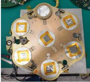
The focal plane structure holding 7 X-ray cameras. The thin (square) filters that protect each hard X-ray camera are visible, along with a photocell used for alignment (at left). The soft X-ray camera (at top) has a special, circular filter that is much thinner than the others to allow the transmission of low-energy X-rays.
