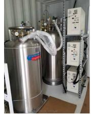
launch. The system was developed for use on remote campaigns where supply chain logistics makes delivery of LN2 difficult, expensive, or impractical.
