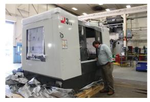
HAAS VF 3 YT vertical machining center.
