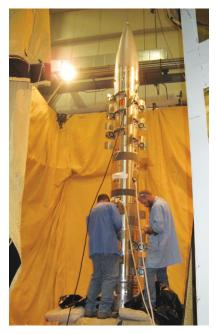
C-REX payload with doors deployed.
