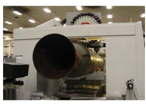
Taurion motor casing being modified in the machine shop.
