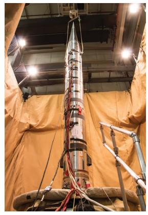
The Sub-TEC 6 payload during deployment testing at Wallops.
