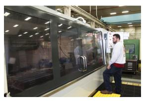
HAAS VF11 vertical machining center.
