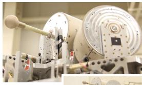
ASSP payload section with subpayloads installed (right). ASSP subpayloads (above).
