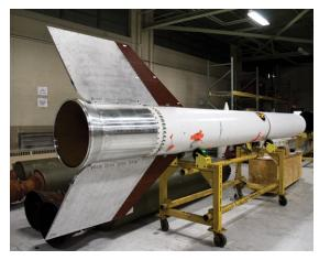
Peregrine motor casing with two of four fins installed for load testing.
