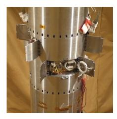
Ampoules visible in payload after door deployment.
