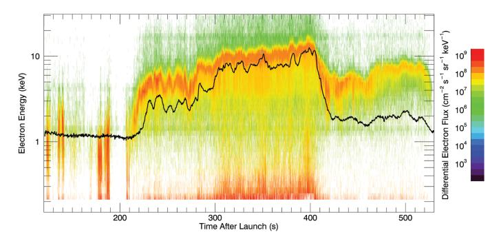
APES instrument electron spectra closely matching ground based auroral signature at the magnetic footprint of the rocket (black line).
