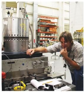
Rocket motor going through vibration testing inside a vacuum chamber.
