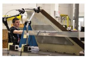
NSROC Testing and Evaluation group intern, Seth Austin, conducting a fin bend test.
