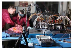
Vibration testing of the WFF Avionics Pallet for LDSD.
