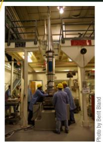
Murbach payload on the vibration table ready for testing.
