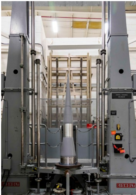
MesOrion 9-inch payload in spin/balance facility at Wallops. Photo by Berit Bland/NSROC
