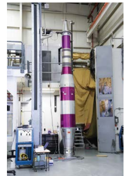
Bend testing of payload. Photo by: Berit Bland/NSROC
