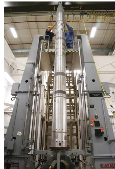
Payload being prepared for balancing. Photo by: Berit Bland/NSROC
