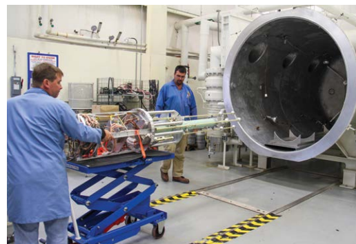
Payload ready to enter the thermal-vacuum chamber. Photo by: Berit Bland/NSROC
