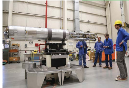
Payload placed on mass properties measurement table. Photo by: Berit Bland/NSROC
