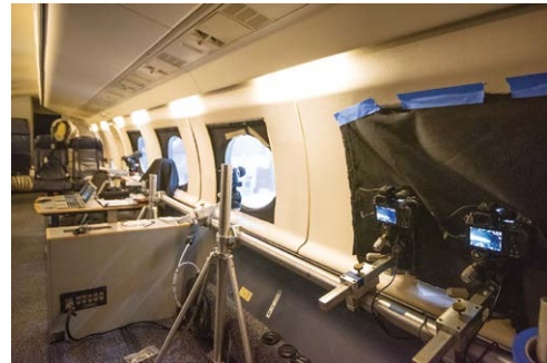
Camera setup onboard aircraft to image vapor tracers. Photo by: Dr. Conde
