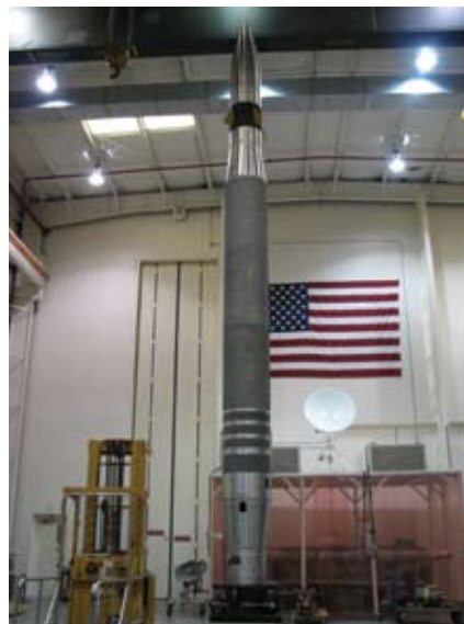
MARTI payload on mass properties table.
